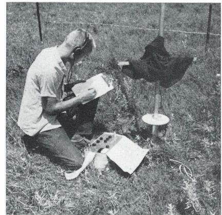
Using a permanent antenna to determine the direction of a radio "bugged" prairie chicken.
