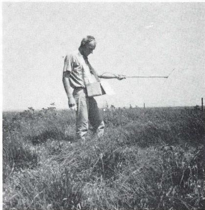
A portable receiver and hand held antenna or electronic "bird dog" being used to pinpoint or flush a radio-tagged prairie chicken.
