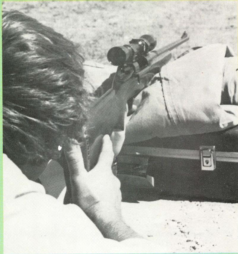
Bore sighting a rifle. The barrel is lined up with a nearby target. Then the rifle is held steady while the sights are adjusted.
