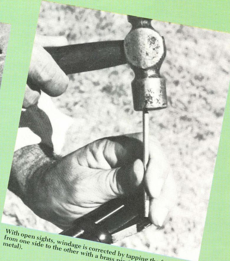
With open sights, windage is corrected by tapping the front sight from one side to the other with a brass pin (to avoid marking the metal).
