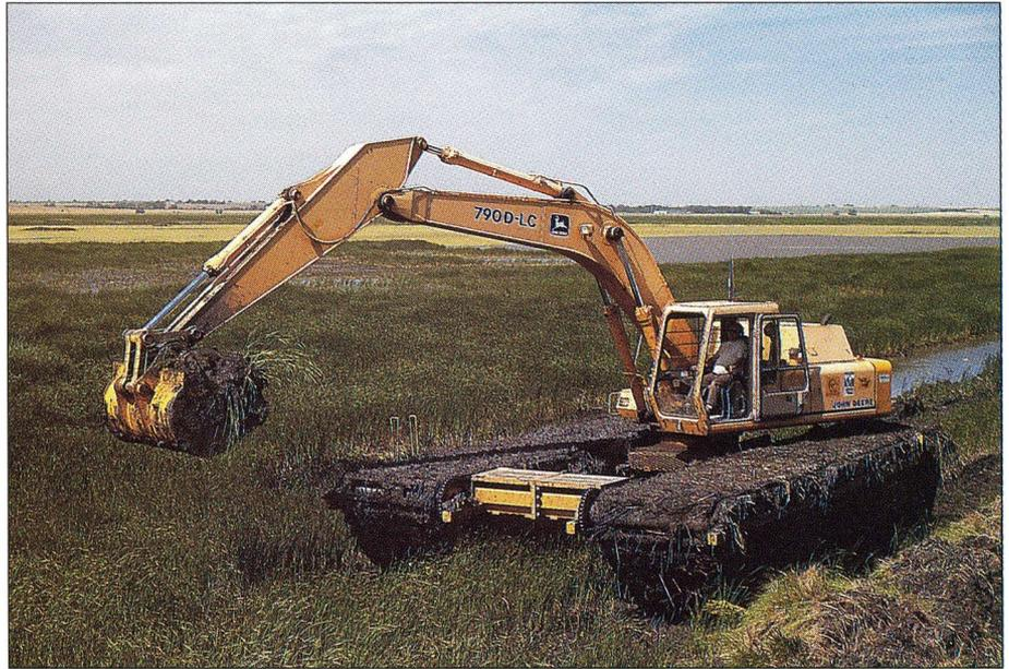
The department's amphibious backhoe is used to dig the level ditches, which will hold deep water for storage and create additional wildlife habitat.
