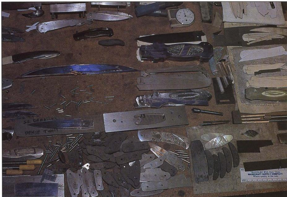
All Herman knives are original designs. However, he may make several knives based on one general design, pre-cutting components prior to final assembly and finish.
