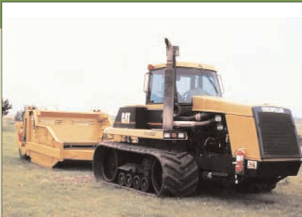
Cheyenne Bottoms renovations have allowed managers to move water more efficiently and dry pools for cattail control. However, acquisition of specialized equipment such as a tracked tractor (with scraper attached above) and large discs is also critical to successful management.
