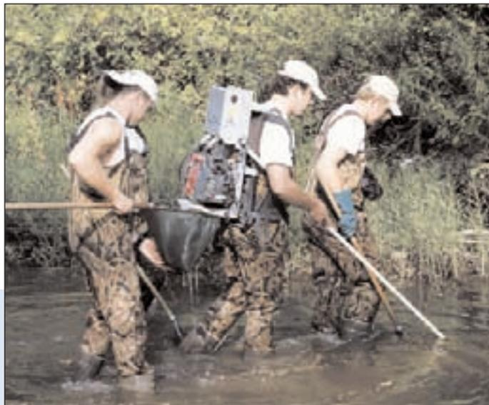
Stream crews sample wadable streams and rivers using equipment such as the backpack electroshocker, above.
