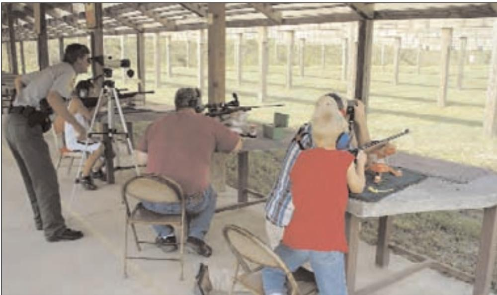
Covered shooting lines and baffles can prevent bullets from being fired in an unsafe direction. Downrange, a berm with bullet catchers stop all bullets.
