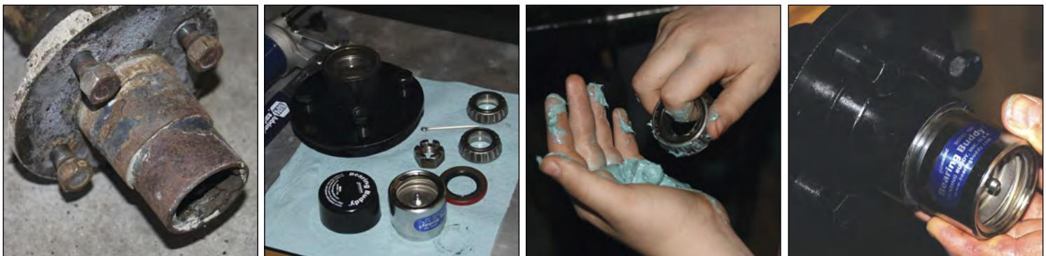
Repacking wheel bearings and installation of new bearing buddies and seals will help ensure a longer life for the trailer, and hopefully prevent breakdowns during fishing trips. Hunter enjoyed working in the grease, but it was only four bearings. The final result was quite a change from what we started with. Below, Hunter uses a angle grinder to remove heavy rust on the outside of the channel iron frame.
